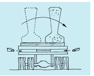
In some cases, beams are delivered side by side by tractor and rear bogie rig. It is important to chock the turntables of the loads before the first beam is lifted as otherwise the second beam would apply an eccentric load to the bogie and cause it to rotate.
