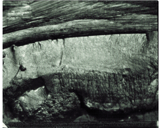
Figure 32: Seaward left outer weld stub axle - beach marks
