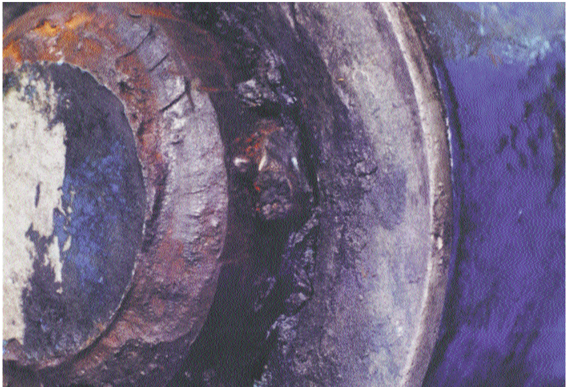
Figure 15: Seaward right stub axle - fracture surface - seized in support foot
