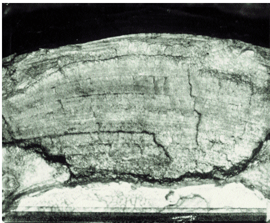
Figure 33: Seaward left inner weld stub axle - beach marks
