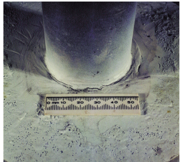
Figure 24: Shore end right stub axle/collar joint from below - fatigue cracks
